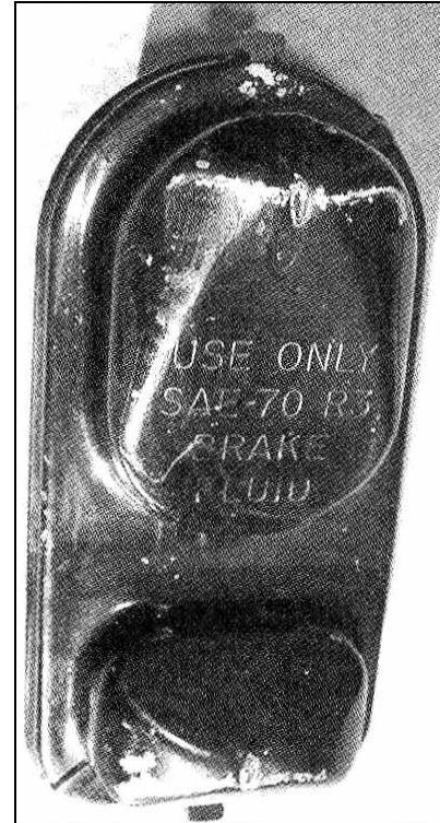
6. Filler caps on disc brake master cylinders manufactured prior to the introduction of the 1970 models in 1969 were stamped "USE ONLY SAE-70 R3 BRAKE FLUID" (right). Starting with the 1970 model line the brake fluid information stamped on disc brake caps was changed to "USE ONLY SAE J1703 BRAKE FLUID" (left). In 1972 information pertaining to brake fluid was removed altogether.
