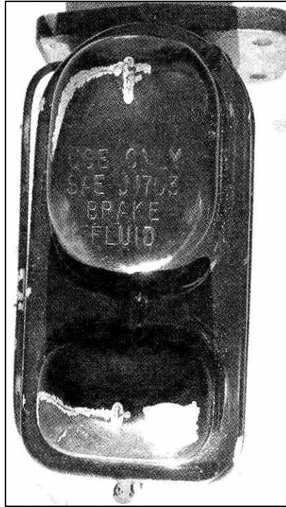
6. Filler caps on disc brake master cylinders manufactured prior to the introduction of the 1970 models in 1969 were stamped "USE ONLY SAE-70 R3 BRAKE FLUID" (right). Starting with the 1970 model line the brake fluid information stamped on disc brake caps was changed to "USE ONLY SAE J1703 BRAKE FLUID" (left). In 1972 information pertaining to brake fluid was removed altogether.
