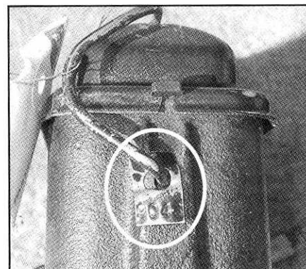
5. Disc brake master cylinders manufactured prior to mid-1969 have a bail wire tag which contains date code information. This example, reading "9043", was manufactured on the 43rd day of 1969.
