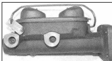
10. The most common disc brake master cylinder is the 3461176, which was installed on B-, C-, and E-body cars from 1971 through 1975. 3461178, which was installed on many A-bodies, uses the same casting and is identical other than minor internal piston stroke differences. Note that there's no piston retainer screw or boss. '75-up masters were similar to this, but a tad larger-until the changeover to aluminum 2-bolt units that began in 1979.
